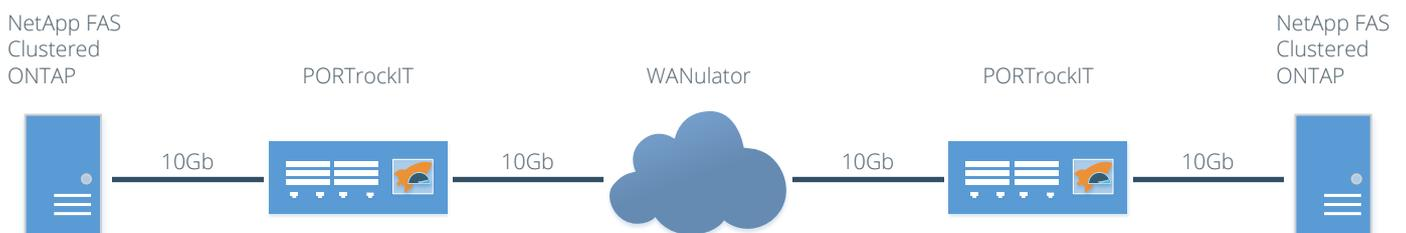
**Figure 2:** Accelerated architecture with PORTrockIT
