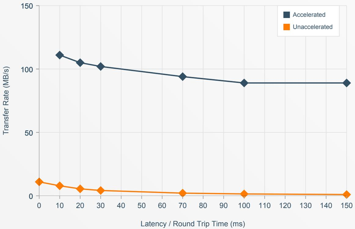
Figure 5: Accelerated and unaccelerated performance with 1% packet loss at various levels of latency
