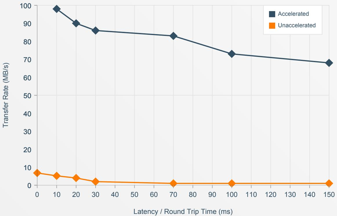
Figure 6: Accelerated and unaccelerated performance with 1.5% packet loss at various levels of latency
