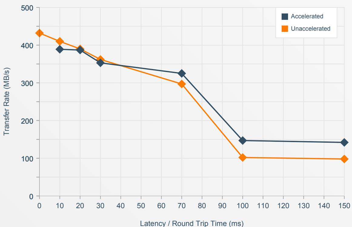
**Figure 3:** Accelerated and unaccelerated performance at various latencies with 0% packet loss
