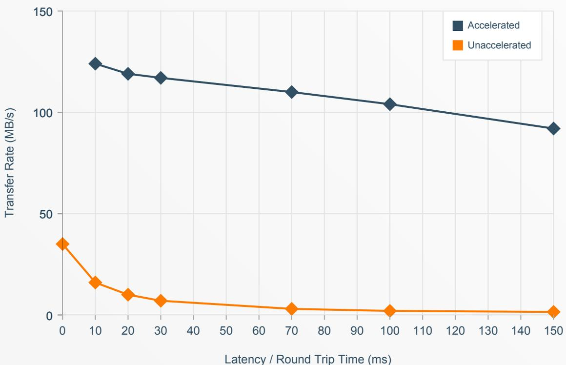
**Figure 4:** Accelerated and unaccelerated performance with 0.5% packet loss at various levels of latency
